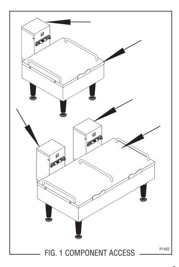
The receptacle cover is attached with four #6-32 truss head locking screws.
