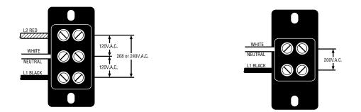
These brewers require either 3-wire, grounded service rated 120/208 or 120/240 volts ac or 2-wire, grounded service rated 200 volts ac, or 20 amp, single phase, 60 Hz. Refer to the product's data plate above the dilution nozzle for actual voltage of your particular brewer model.
