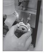
Twist Whipper Chamber Receptacle clockwise and pull it off the Motor Shaft.
