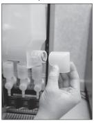
3. Pull the Ejector Elbow off the Hopper Base.
