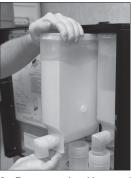
2. Remove the Hopper/ Base Assembly from the Cabinet. Remove the Cover and empty the contents.
