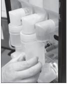
3. Pull the Mixing Chamber out of the Whipper Chamber.
