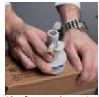
10. Remove the mating end of connector and attach dispenser's connector to a Bag In a Box and dispense several cups to prime the concentrate line or until consistancy of the product is correct. If using bottled concentrate, replace the draw tube in the concentrate bottle.
