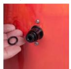
7. When finished, slide the o-ring back into the groove on the venturi nozzle.
