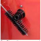
6. Clean the groove and o-ring with the same solutions as used to clean the faucet. Step 8.
