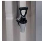
Unscrew the faucet 4. Twist the faucet wing nut in a clockwise direction and remove faucet from the dispenser.
