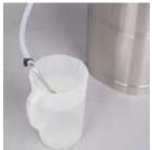
If using bottled concentrate, place the draw tube in the container with soap solution.
