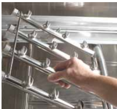
One-Piece Cast Stainless Steel Spray Assembly
