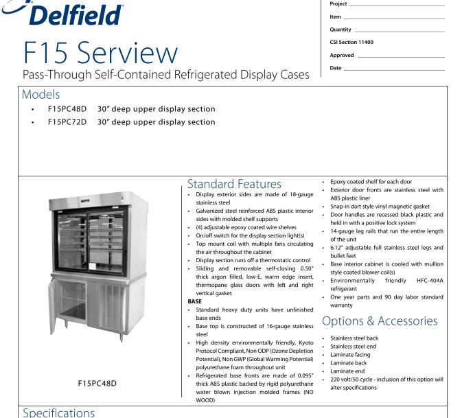
Top is constructed of 16-gauge stainless steel, with integral front and rear nosing. Interior sub-top is made of ABS plastic and 2.00° die foam is laminated between the interior and exterior top.
