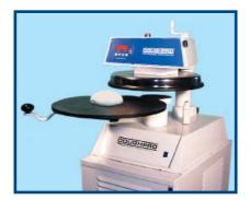
After allowing upper platen to reach desired temperature, swing out lower platen and place pre-portioned ball of dough in approximate center and swing closed. An approved lubricant/release agent such as olive oil or DOUGHPRO's Cookware Food Release Spray #DPPC1 applied to the top of the dough ball will greatly improve the pressing operation.
