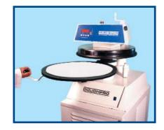
Open platen and place flattened crust on screen, disc or pan. Now you're ready for make-up and baking.
