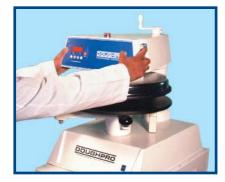
Set the desired time cycle. Push down both left and right compression activation buttons, hold until resistance is felt and release. The DP1300 will automatically release when the time cycle is finished.
