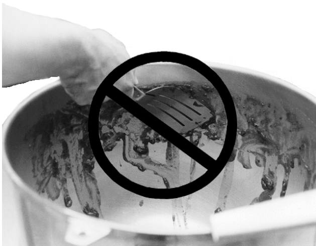
Scrapers, steel wool or metal implements can harm the kettle surface.
