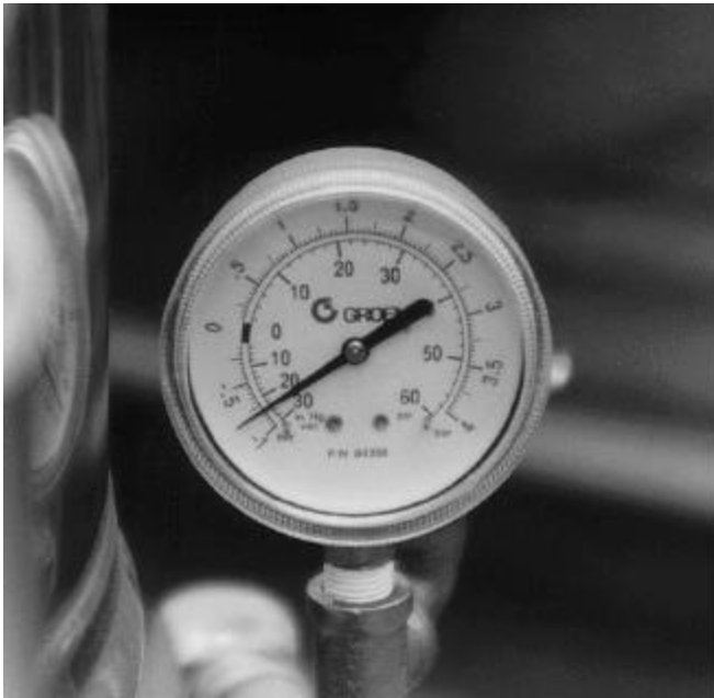
The pressure gauge should show a vacuum of 20 to 30 inches when the kettle is cold.
