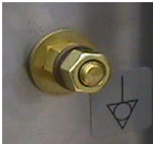
The equipotential terminal is located on the left rear of the HY-3E
