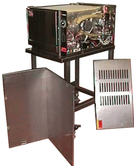
Figure 1 - Remove covers from existing (lower) unit.
