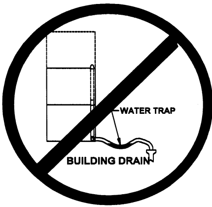
IMPROPER DRAIN LINE CONNECTION
