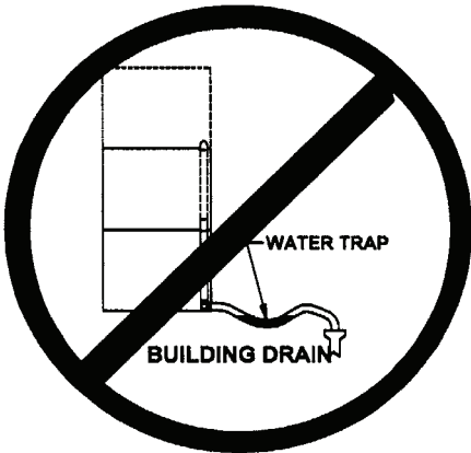
IMPROPER DRAIN LINE CONNECTION
