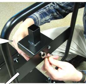
BOLT BRACKET TO HANDLE WITH BOLTS PROVIDED AND SLIDE PUMP AND TUBE ASSEMBLY THROUGH SQUARE TUBES.
