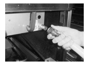
1. Roll disposal shuttle to front of fryer and disconnect shuttle hose from either the male or female fitting, depending upon the matching fitting on fryer.
