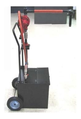
10. Once shuttle is empty, loosen thumb screw on bracket and swivel pump assembly back over lower unit and tighten handle.
