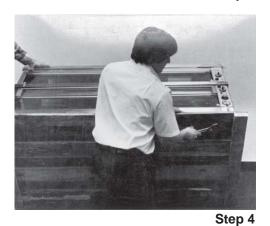
4. Remove four bolts from under skid.
