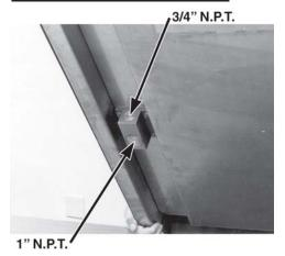
The drain can be connected to a 1 inch N.P.T. directly below the water well or to a 3/4 inch N.P.T. from the operator's side. We recommend the 1 inch N.P.T. connection as this will allow straight down draining of the water.
