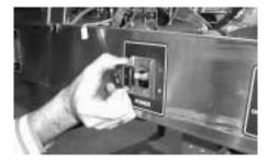
Place the power switch in the off position, and remove power to the fryer by unplugging the unit or turning off the wall circuit breaker. Failure to do so could result in electrical shock.
