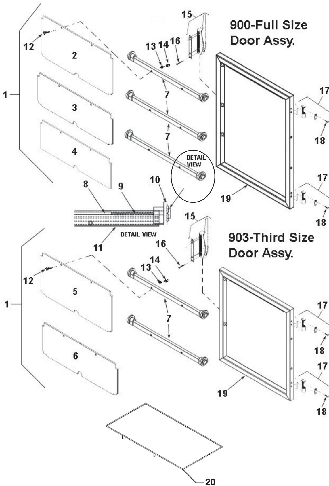
Figure 3-3. Flip-Up Door Assemblies (HHC-903 - SN: DA0511040 & Above)
