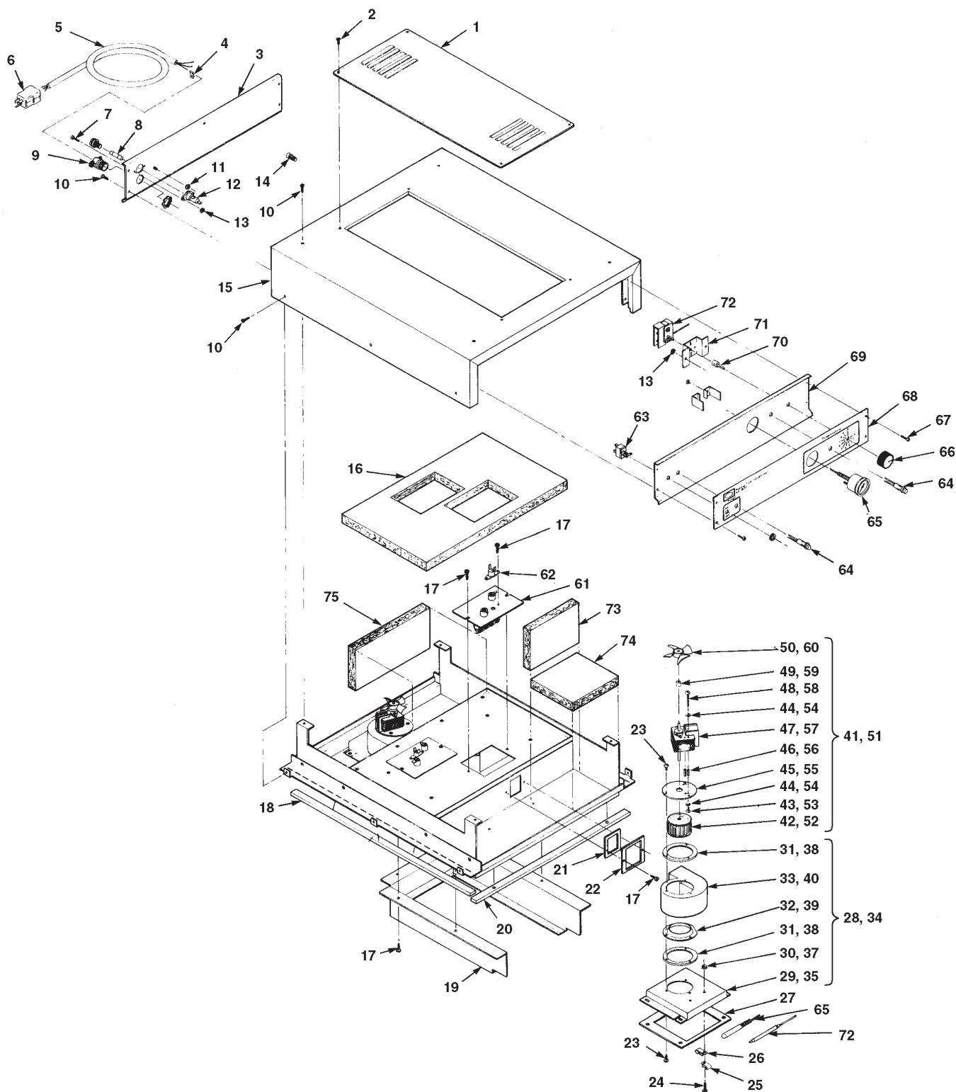
Figure 3-1. Control Module Assembly - UL & CE Approved
