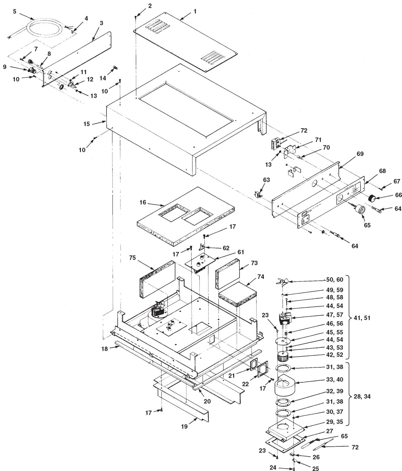
Figure 3-4. Control Module Assembly - Non-UL, Non-CE
