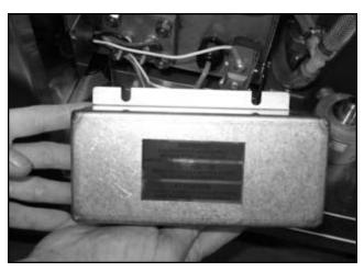
Removing the heater cover.
