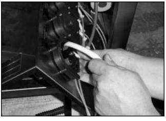
Pulling the rubber tube out of the pump.
