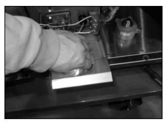
Removing the lower strainer.
