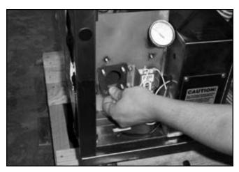
Removing the heater gasket
