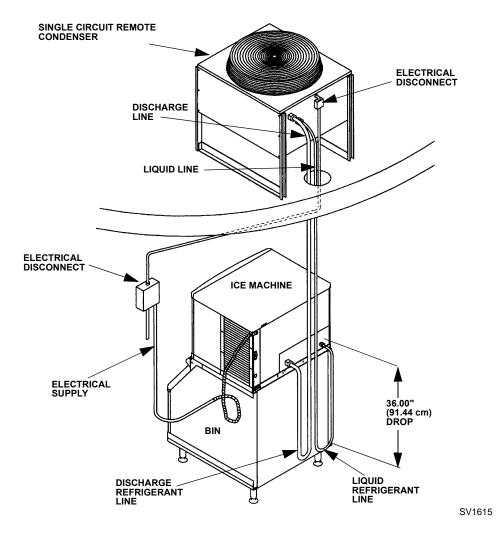
Figure 2-10. Typical Single Circuit Remote Condenser Installation
