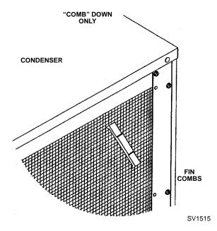
Straighten Bent Condenser Fins
