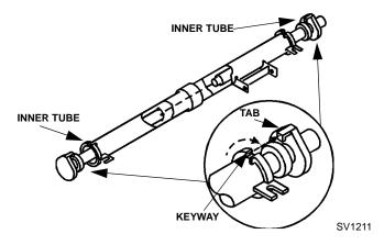
Water Distribution Tube Disassembly
