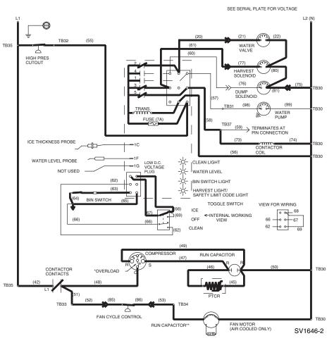
Figure 6-2. Self-Contained — Refrigeration System Start-Up
