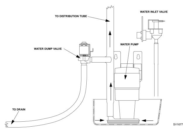
Figure 5-1. Water Flow Over the Evaporator
