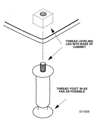
Figure 2-1. Leveling Leg and Foot
