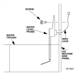
Water Level Probe Removal
