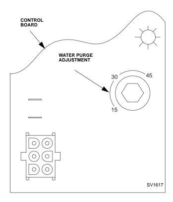
Figure 3-10. Water Purge Adjustment
