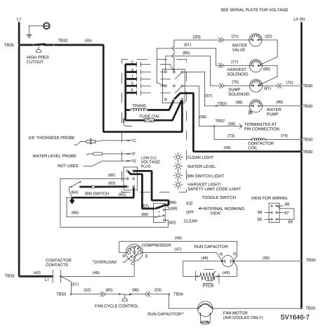
Figure 6-7. Self-Contained — Automatic Shut-Off
