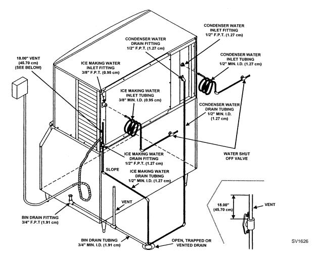
Figure 2-3. Typical Water Supply Drain Installation
