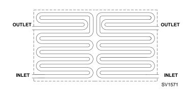
Figure 7-11. Q1300/Q1600/Q1800 Evaporator Tubing
