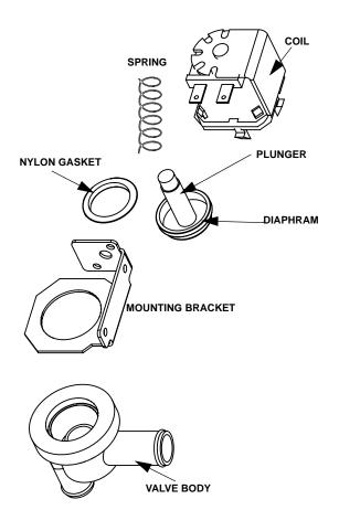
Dump Valve Disassembly
