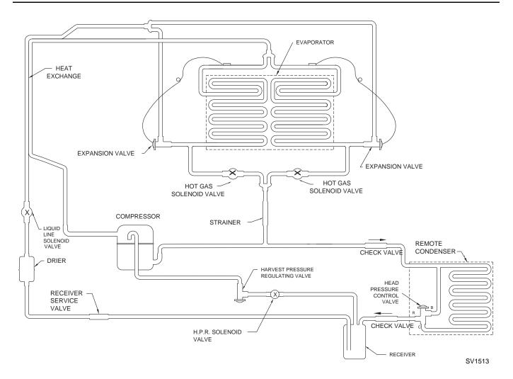
Figure 7-7. Q1300/Q1600/Q1800 Remote Models
