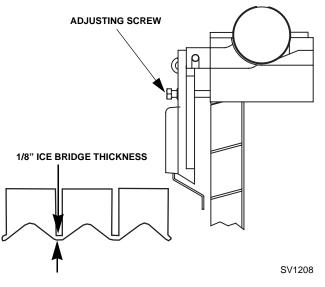
Figure 3-9. Ice Thickness Check
