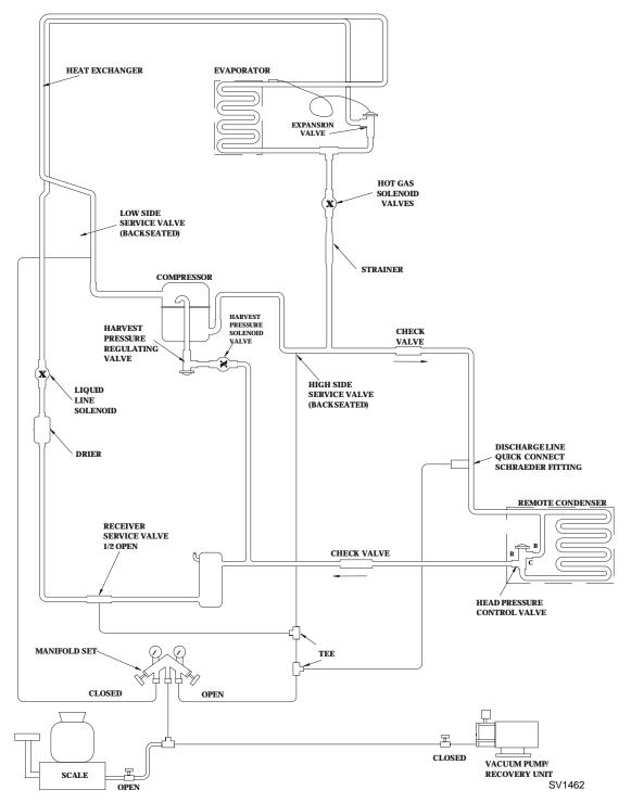
Figure 7-17. Remote Charging Connections
