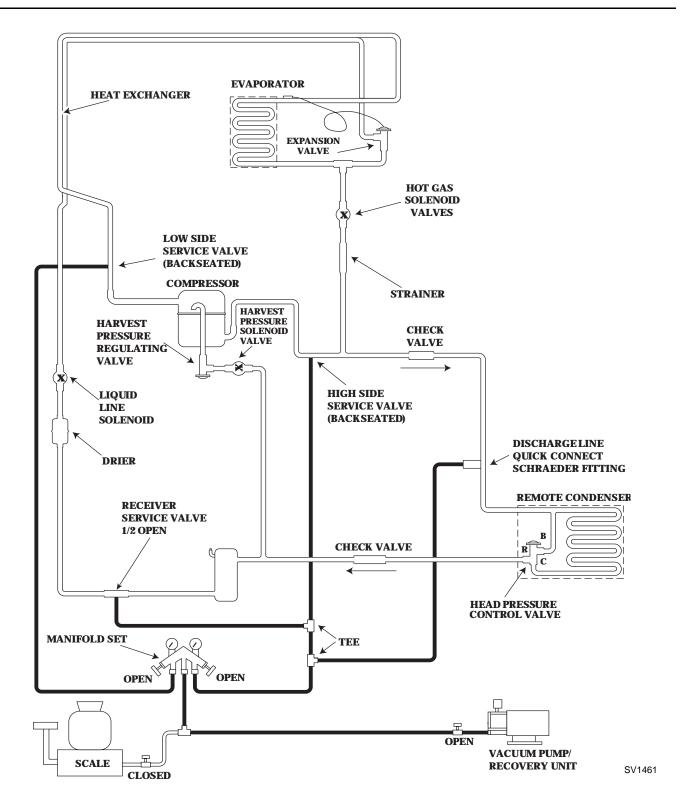
Figure 7-16. Recovery/Evacuation Connections
