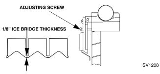
Figure 6-21. Ice Thickness Check
