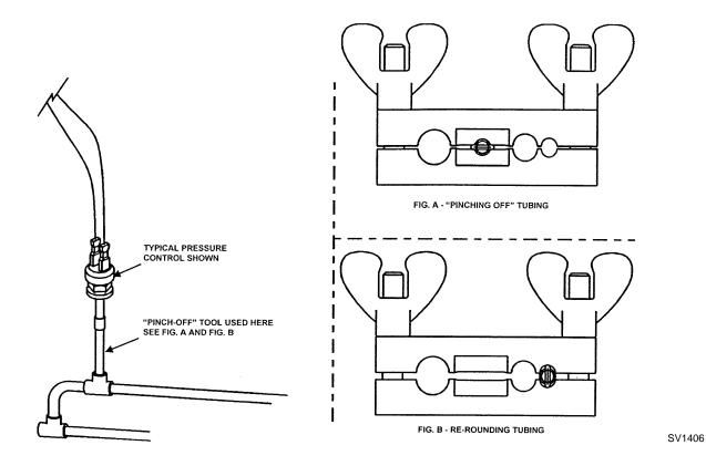
Figure 7-18. Using Pinch-Off Tool
