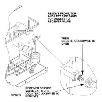
Figure 2-9. Backseating the Receiver Service Valve
