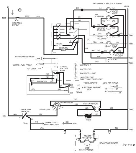
Figure 6-9. Remote — Refrigeration System Start-Up
