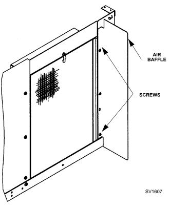
Figure 2-2. Air Baffle
