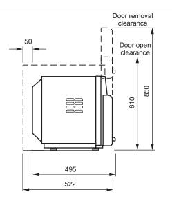
Allow a minimum of 50mm clearance to sides, top and rear to allow air to circulate freely
