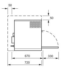
Allow a minimum of 50mm clearance to sides and rear to allow air to circulate freely
