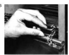
To reassemble, reverse the procedure. Be sure to reassemble the belt with the knuckle opening facing away from the direction of travel.
