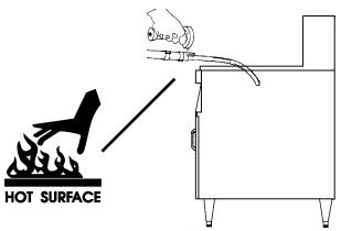
13. Turn fryer on and make sure thermostat is set to your cooking temperature. Using fresh shortening carefully refill fryer to proper level. A small amount of shortening will be left in the filter tank, which is normal.
