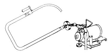
IMPORTANT: This hose is flexible. However, excessive bending can crease or crack the hose causing hot oil to leak. Do not use a creased or cracked hose.
