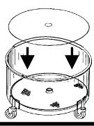
IMPORTANT: Center paper properly so it lays flat on screen and overlaps on each end. If incorrect, torn or no filter paper are used, the unit will not filter properly.
