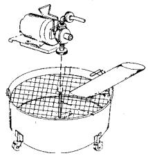
9. Attach anti-splash tube on the filter tank by hooking the tube over the rim of the tank so the diffuser end of the tube is closest to the safety quard. (See drawing above)
