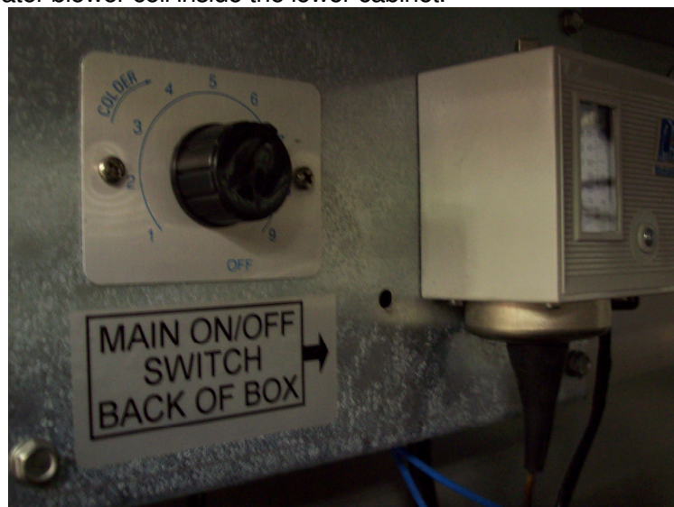
Figure 1 illustrates the electrical control box inside the mechanical compartment. The on/off switch for the rail is located on the front of the control box while the main on/off switch for the entire unit is located on the rear of the control box. The thermostat adjustment knob for the upper rail is located on the side of the control box. (This thermostat also controls the refrigerated catch pan area).
