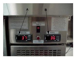
**Figure 1** illustrates the outer panel of the mechanical housing. Item **A** is referencing the temperature control for refrigerated rail, and Item **B** is referencing the temperature control for the refrigerated base.
