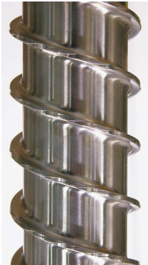
Example of a Clean Auger
