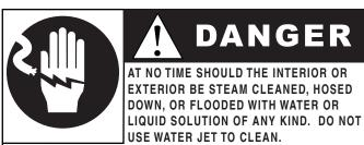
SEVERE DAMAGE OR ELECTRICAL HAZARD COULD RESULT.
