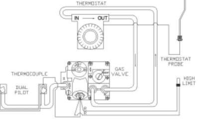
Figure 1. Fryer Model 14GS Wiring Diagram
