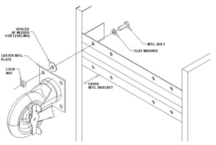
Figure 4. Typical Caster Installation
