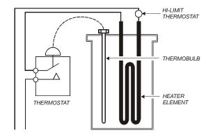
Fig. 3 Heat Control Diagram
