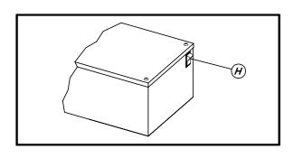
H. TANK HEATER SWITCH ALLOWS MAIN TANK HEATING ELEMENT TO BE TURNED OFF OVERNIGHT OR DURING SLOW PERIODS
