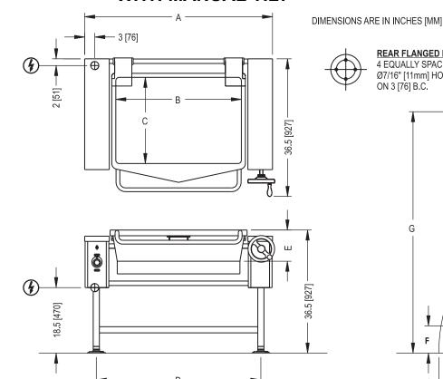
**REAR FLANGED FOOT DETAIL** 4 EQUALLY SPACED Ø7/16" [11mm] HOLES ON 3 [76] B.C.
