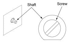
Calibrate the thermostat by holding the shaft in place while turning the screw counterclockwise to increase the temperature, or clockwise to decrease the temperature.
