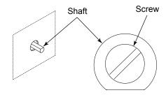
Calibrate the thermostat by holding the shaft in place while turning the screw counterclockwise to increase the temperature, or clockwise to decrease the temperature.
