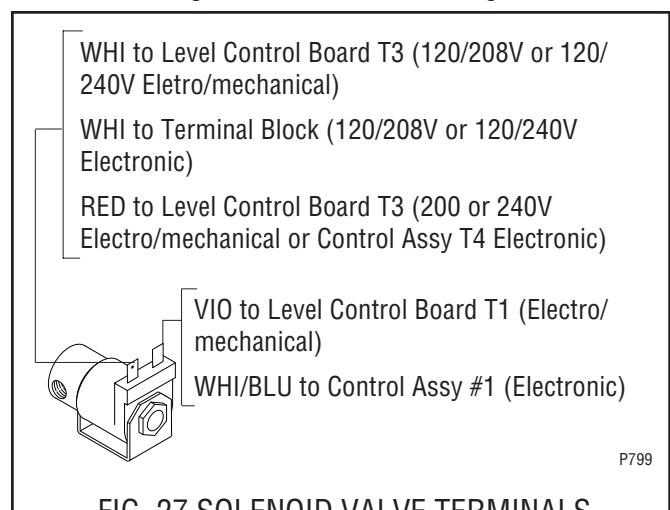
FIG. 27 SOLENOID VALVE TERMINALS
