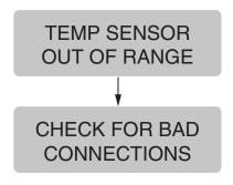
1. Temperature Sensor Probe wire(s) broken or not making connection.
