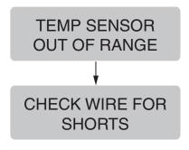
1. Temperature Sensor Probe wire(s) shorted to housing, or to each other.
