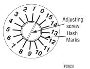
Turn the adjusting screw counterclockwise to the desired setting as noted below.
