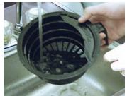
Clean and sanitize the funnel. 2. NOTE: Do NOT clean this equipment with a water jet device.
