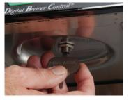
Use the blunt end of sprayhead cleaning tool to clean the sprayhead outlet fitting.
