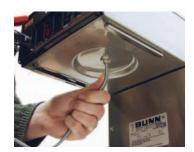
With the sprayhead removed, insert a deliming spring into the sprayhead tube until approximately two inches of the spring remain visible. Saw back and forth five or six times to loosen any lime deposits.
