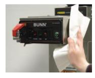
Use a clean damp cloth rinsed in mild, non-abrasive detergent to clean all outer surfaces.
