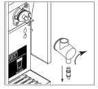
4. Twist the Whipper Chamber clockwise and pull it off the Whipper Chamber Receptacle.
