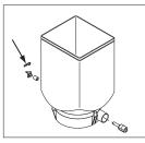
6. Remove the Auger Drive Shaft by removing Retaining Clip from Auger Drive Shaft.
