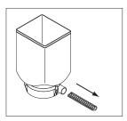
5. Remove Auger by pulling it out the front of Hopper Base.
