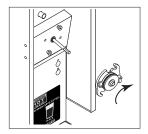
6. Twist Whipper Chamber Receptacle clockwise and pull it off the Motor Shaft.
