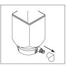
3. Pull the Ejector Elbow off the Hopper Base.
