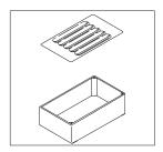
1. Empty the Drip Tray and wash components in a mild solution of dish detergent using a bristle brush. Rinse and dry each item thoroughly before reassembling.
