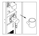
3. Pull the Mixing Chamber out of the Whipper Chamber.
