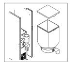
2. Remove the Hopper/ Base Assembly from the Cabinet. Remove the Cover and empty the contents.
