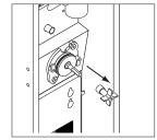
5. Pull the Frother off the Motor Shaft. Notice the flat keyway on the shaft and the matching keyway inside the Frother. It is important that these two keyways are lined up when reassembling.
