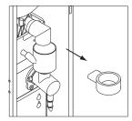
2. Remove the steam collector by pulling it forward and twisting in a clockwise rotation.
