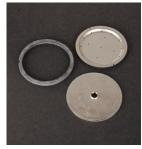
STEP 5 Remove the gasket to separate the two halves. Clean and sanitize all parts. Verify all the holes are open.
