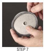
Install gasket around the assembled sprayhead. Reinstall spravhead on brewer.
