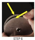
To reassemble sprayhead, align the dimples as shown.
