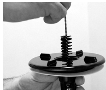
10. Clean the inlet tube with the medium sized brush and the cleaning solution.
