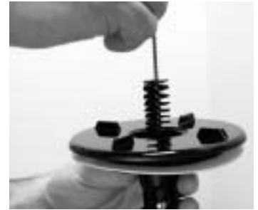
9. Clean the inlet tube with the medium sized brush and the cleaning solution.
