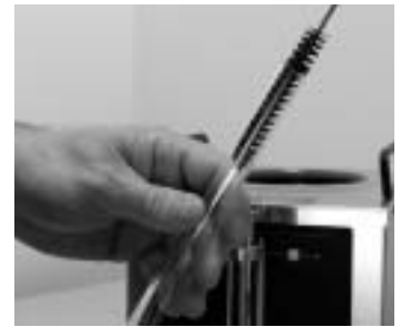
13. Clean the sight gauge with the large brush and reassemble the sight gauge.
