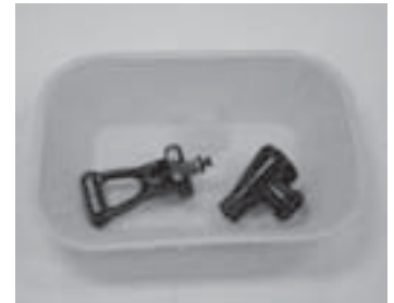
17. Allow the parts to soak in a sanitizer solution for a minimum of ten minutes. Remove the faucet parts from the sanitizer solution and rinse thoroughly. Allow parts to air dry over night.
