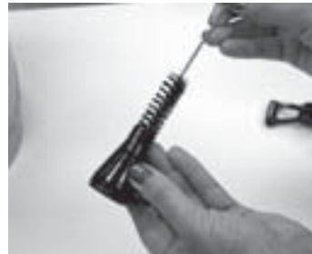
16. Use a small brush (BOM #00674.0000) to thoroughly scrub the faucet body.
