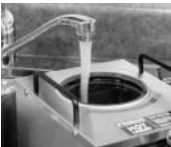
18. Thoroughly rinse the entire inside of the server. DO NOT immerse the server in water.
