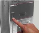
Press and release the "START" switch to begin grinding. Once grind cycle is complete, remove funnel from grinder. Go to step #8.
