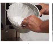
Insert a BUNN<sup>®</sup> filter into the 4. 3. funnel. If no grinder is being used, go to step #7.
