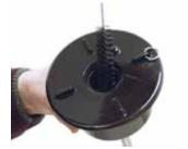
8. Clean the airvent with the small brush provided (26367.0000) using a cleaning product and water solution. Clean the inlet tube with the medium-sized brush and the cleaning product solution.
