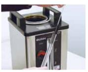
10.Unscrew the sight gauge cap. 11.Clean the sight gauge with the large brush (00675.0000) and reassemble.
