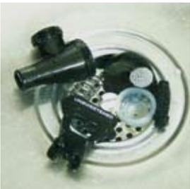
11. Sanitize the parts by soaking for one minute in the warm chlorine solution.
