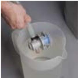
6. Place bag connector into a 1/2 gallon container of dish soap and warm to hot water (130° F/54° C).
