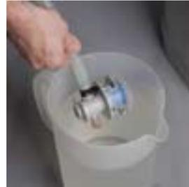
14. Sanitizing the BIB connector, tubing and metering valve: This procedure requires a 1/2 gallon container of sanitizing solution, (100 ppm of chlorine at 100° F (38° C) water).
