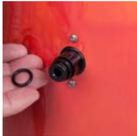
7. When finished, slide the o-ring back into the groove on the venturi nozzle.
