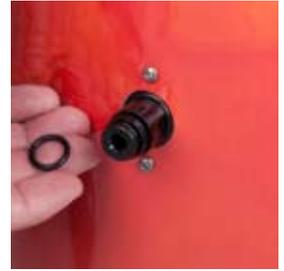
5. Remove the o-ring from the venturi assembly nozzle. Be very careful when removing this o-ring. Do Not scratch or nick the o-rings sealing surface when removing.
