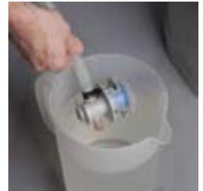
9. After the soap mixture has been flushed through the system, fill the container with warm to hot tap water only (no soap) and repeat steps 6 thru 8 until all soap has been flushed from the system.
