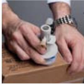
3. Since the bag connector(s) have an internal shut off built in, it will be necessary to cut off mating end of a Bag In a Box. Keep this mating end for future cleanings of the system.
