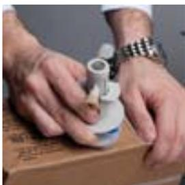
10. Remove the mating end of connector and attach dispenser's connector to a Bag In a Box and dispense several cups to prime the concentrate line or until consistency of the product is correct. If using bottled concentrate, replace the draw tube in the concentrate bottle.
