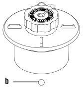
2. Completely disassemble the lid assembly for cleaning by removing the inlet tube assy (a) and inlet ball (b) from the bottom of the assembly. (See illustration at left.) The inlet tube assy is removed by unscrewing it in a counterclockwise direction.
