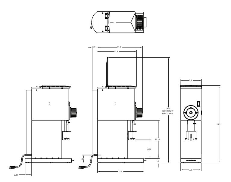
OPTIONAL: BASE CAN BE MOUNTED WITH OFFSET AS SHOWN FOR ADDITIONAL BAG CLEARANCE.
