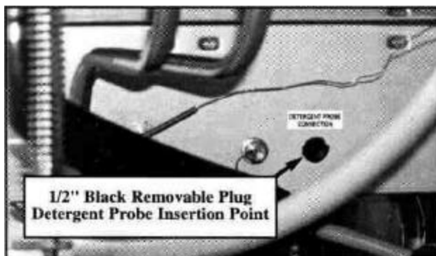
Figure 5 D-HB, D-H1, D-LF Detergent Probe Insertion Point Wash Tank (Rear)
