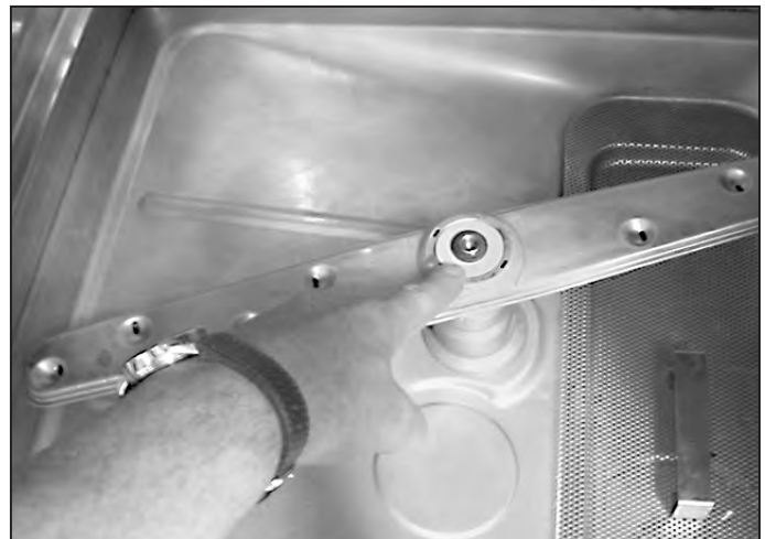
Clean the upper and lower wash spray arm bearings.
