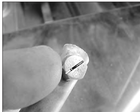
Clean the final rinse arm nozzles.
