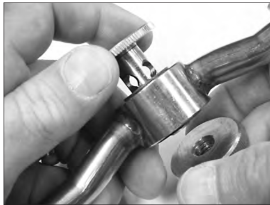
Disassemble the rinse arm assembly.
