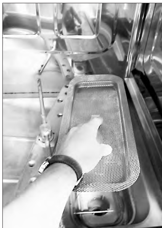
Make sure that the scrap screen is in place.
