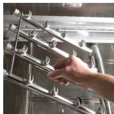
One-Piece Cast Stainless Steel Spray Assembly
