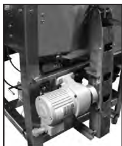
Conveyor oil-free energy efficient drive system.
