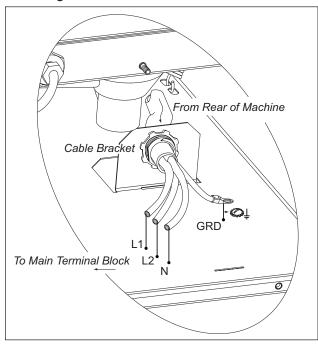
Route the supply cable through the cable bracket.
