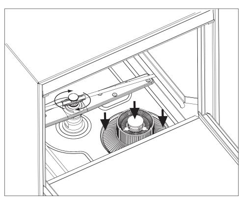
Install the scrap screen, overflow tube, and spray arms.
