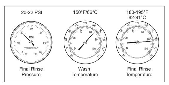
The pressure and temperature gauges are located on the lower-left corner of the lower-front access panel.
